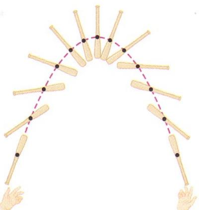
The center of mass of a body or a system of bodies is the point that moves as though all of the mass were concentrated there, and all external forces were applied there.
